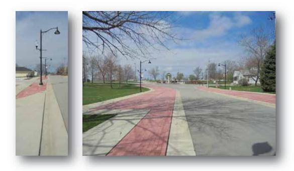
The Village of Dieterich recently replaced deteriorated non-ADA sidewalks along Main Street and Virginia Street which had become a hazard to pedestrian traffic. The new decorative ADA-compliant sidewalks feature a red stamped concrete treatment, curbs and gutters, and decorative lighting. Not only did the sidewalk replacement reduce the hazards to pedestrian traffic, it enhanced the beauty of the downtown business district.
