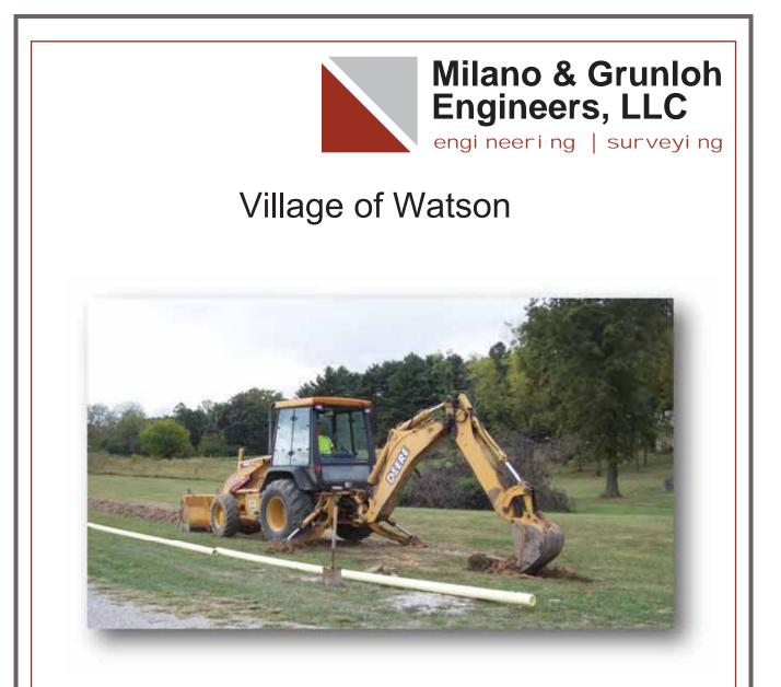
The Village of Watson serves approximately 300 users with 70,000 linear foot of watermain. The Village was experiencing water main breaks and low pressure due to the aging cast iron watermains within their system. Milano & Grunloh Engineers, LLC worked with the Village to develop project areas for the proposed improvements, completed all permitting, applying for grants and loans, and all of the engineering and surveying for the project.
