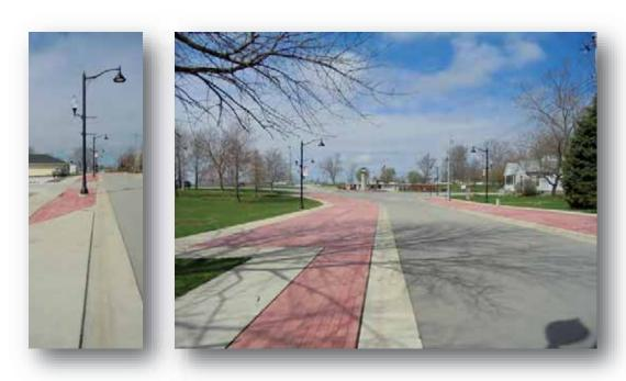
The Village of Dieterich recently replaced deteriorated non-ADA sidewalks along Main Street and Virginia Street which had become a hazard to pedestrian traffic. The new decorative ADA-compliant sidewalks feature a red stamped concrete treatment, curbs and gutters, and decorative lighting. Not only did the sidewalk replacement reduce the hazards to pedestrian traffic, it enhanced the beauty of the downtown business district.
